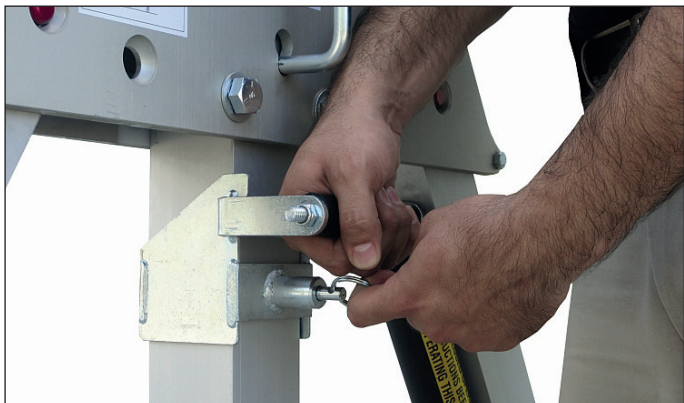
Adjust the mast lift lever with the spring-loaded positioner to a comfortable lifting position.
