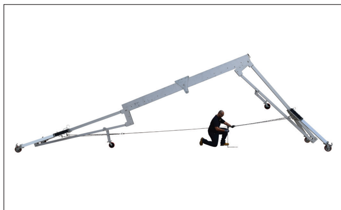
Operate the ratchet on the first A-frame to secure the beam with a pin.
