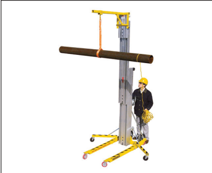
Boom with Mobile Base (Part No. 783642) is ideal for overhead lifting or pipe installation. It features four spring-loaded positioners, 40" / 100 cm reach, and five hook positions supporting 650 - 200 lbs / 300 - 90 kg
