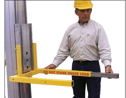
Fork Extensions (Part No. 783691) extend forks from 28 - 42" / 71 - 106 cm at a button press, reducing capacity to 200 lbs / 90 kg. Another button retracts them for internal storage.
